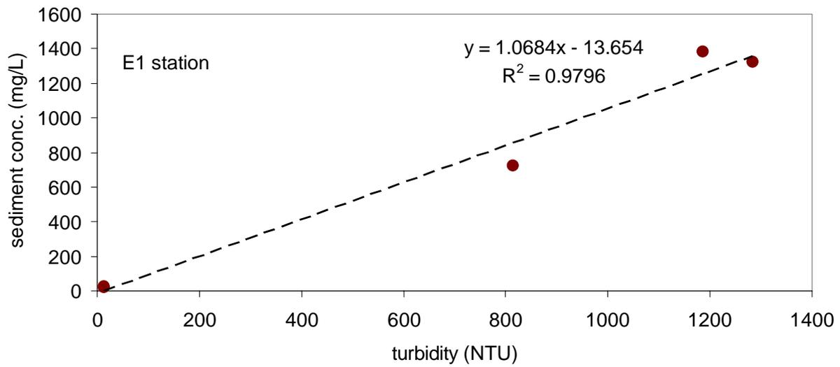
Figure 3.8: Relationship between turbidity (NTU) and suspended sediment concentrations (mg/L) for station E1.
