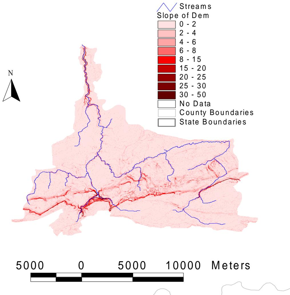
Figure 3.2: Slope gradients (%) in the Eighteen Mile Creek watershed.
