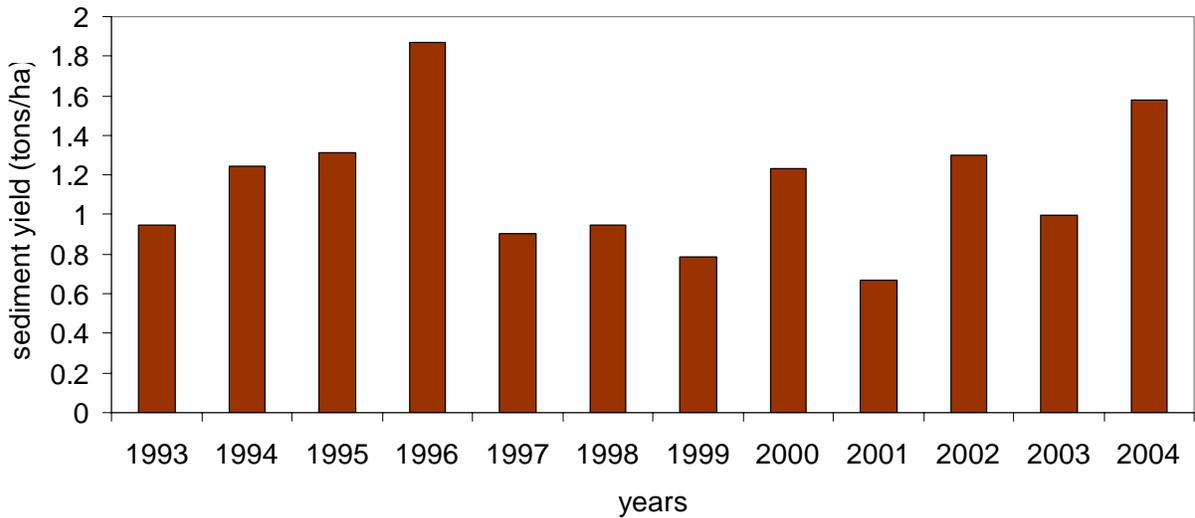
Figure 4.9: Annual sediment yields ( $\text{tons ha}^{-1}\text{yr}^{-1}$ ) for the Eighteen Mile Creek watershed over the 1993-2004 simulation period. Average annual sediment yield was  $1.15 \text{ tons ha}^{-1}\text{yr}^{-1}$ .
