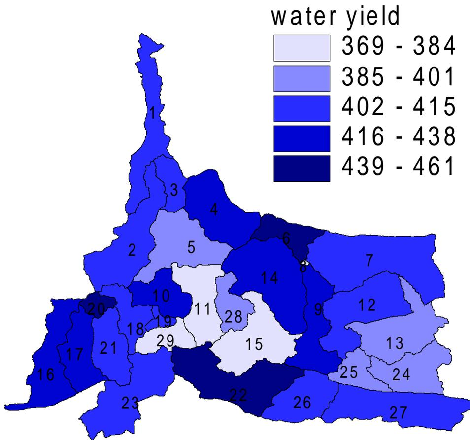
Figure 4.10: Spatial pattern of runoff generation (mm) in the Eighteen Mile Creek watershed.
