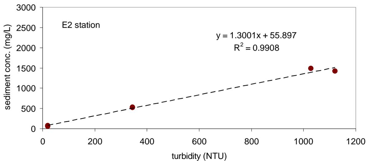
Figure 3.9: Relationship between turbidity (NTU) and suspended sediment concentrations (mg/L) for station E2.
