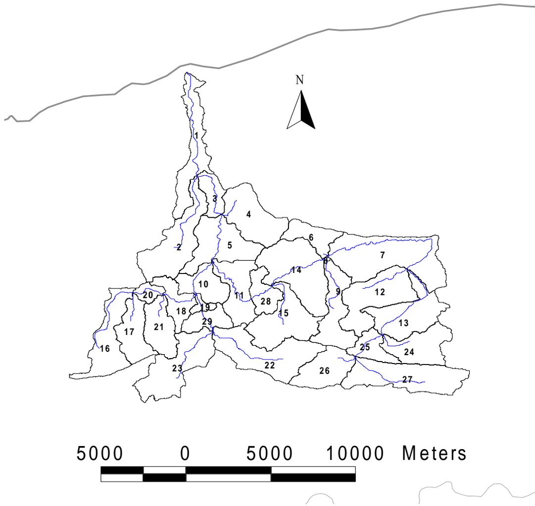
Figure 3.5: SWAT subbasin scheme for the Eighteen Mile Creek watershed.
