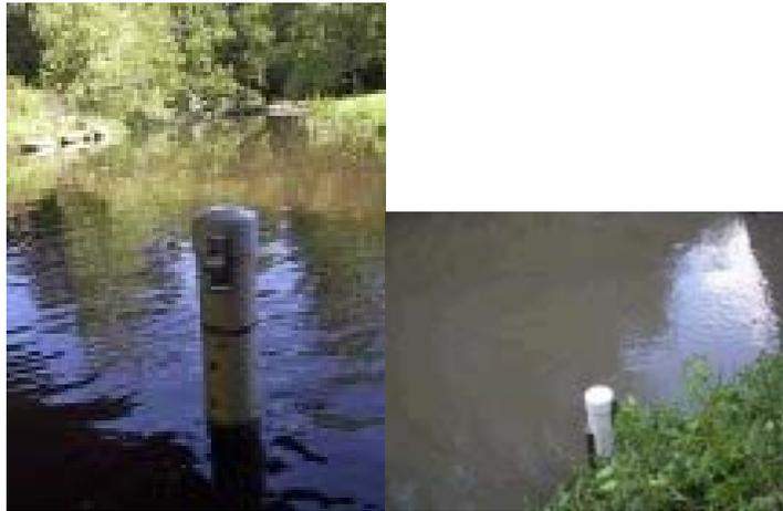
Figure 3.7: YSI sondes located within PVC pipes at stations E1 (left) and E2 (right).
