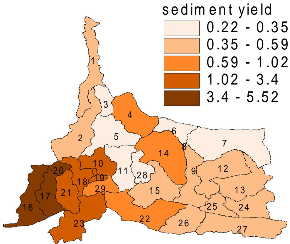
Figure 4.11: Spatial pattern of sediment generation (tons ha<sup>-1</sup>yr<sup>-1</sup>) in the Eighteen Mile Creek watershed.
