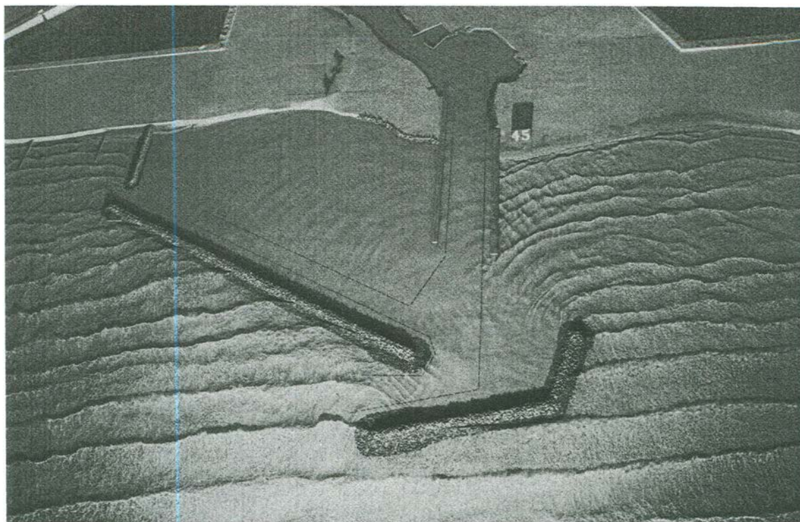
Photo 35. Typical wave patterns for Plan 13; 7-sec, 9.9-ft waves approaching from 343 deg; +2.8-ft swl
