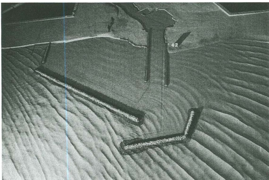
Photo 34. Typical wave patterns for Plan 13; 6.4-sec, 5.B-ft waves approaching from 42 deg; +4.0-ft swl
