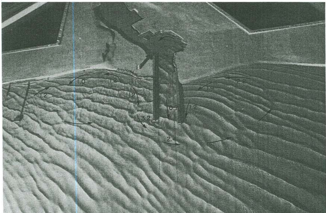
Photo 10. Typical wave patterns, current patterns, and current magnitudes (prototype feet per second) for existing conditions; 6.9-sec, 6.4-ft waves approaching from 42 deg; +2.8-ft swl
