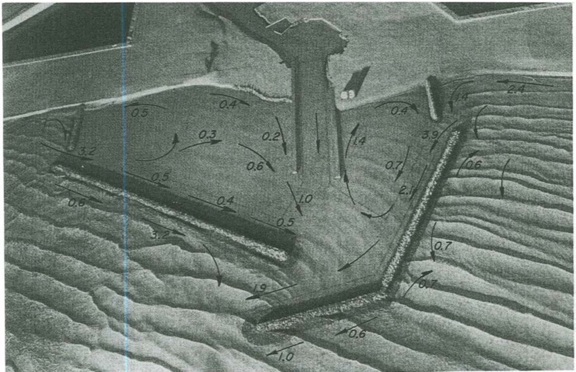
Photo 55. Typical wave patterns, current patterns, and current magnitudes (prototype feet per second) for Plan 19; 6.9-sec, 7.9-ft waves approaching from 24 deg; +2.8-ft swl
