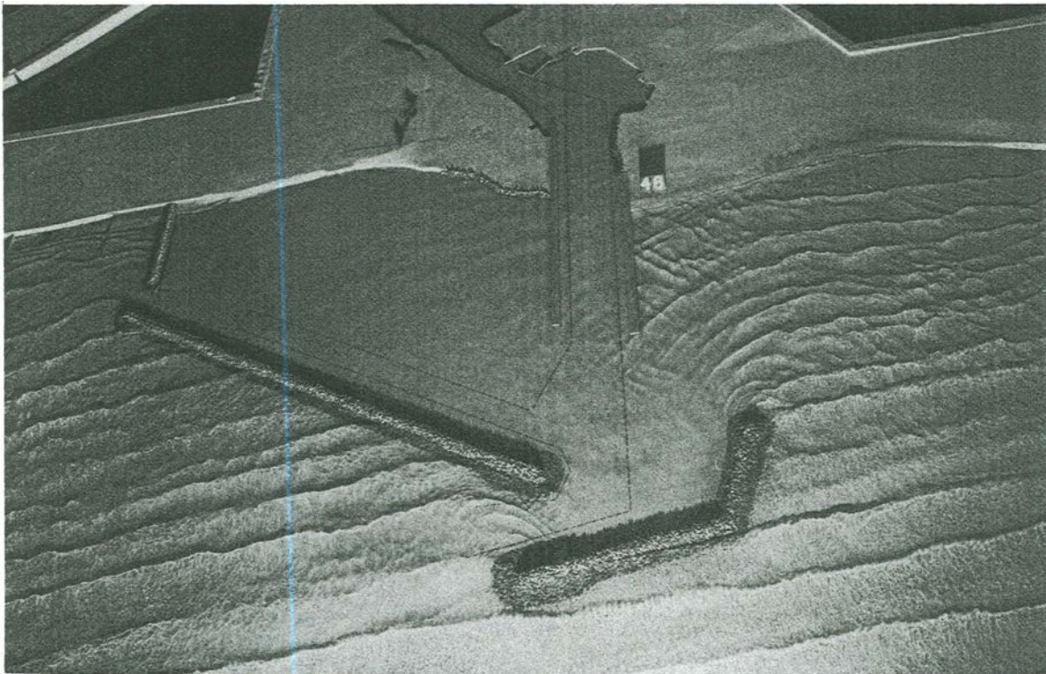
P-10 to 38. Typical wave patterns for Plan 16; 7-sec, 9.9-ft waves approaching from 343 deg; +2.8-ft swl
