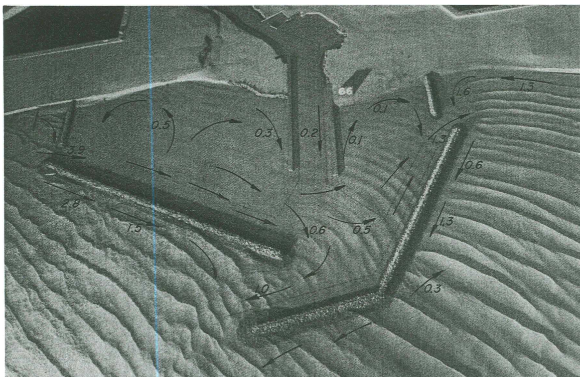
Photo 57. Typical wave patterns, current patterns, and current magnitudes (prototype feet per second) for Plan 19; 6.9-sec, 6.4-ft waves approaching from 42 deg; +2.8-ft swl
