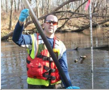
Ben Cole of Ecology & Environment, Inc. collecting a sediment core sample from Eighteenmile Creek.
